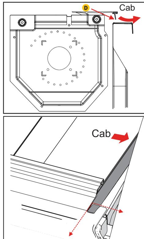
**12 Position the rails:** Move the cover back toward the tailgate and use the shipping bracket as a spacer to position both rails to be 1/8" from the tailgate.
