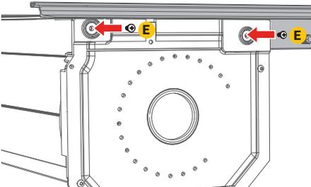
Tighten the canister mounting screws to: 32 in.-lbs.
