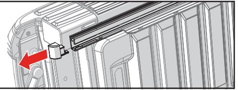
**2 Install the cargo rail mounting hardware:**
